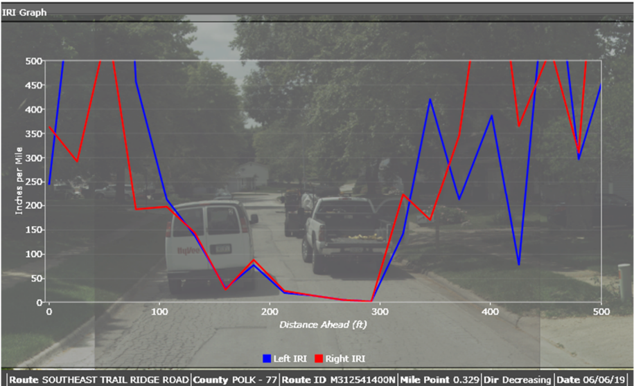
FIGURE 43: ROUGHNESS PROFILE AFFECTED BY LOCAL DRIVING CONDITIONS
