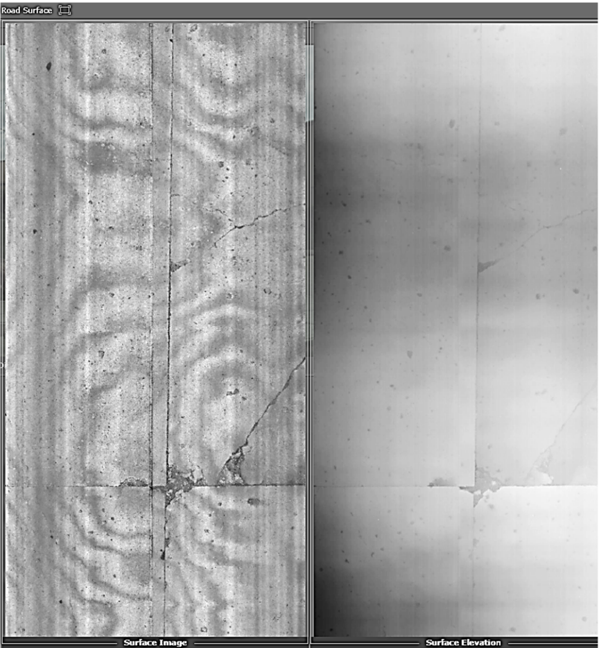
FIGURE 44: UNACCOUNTED FOR PUNCHOUT
