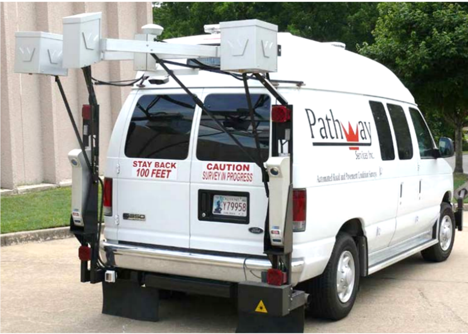
FIGURE 3: A “PATHRUNNER” AUTOMATED DATA COLLECTION VEHICLE (PATHWAYS)
