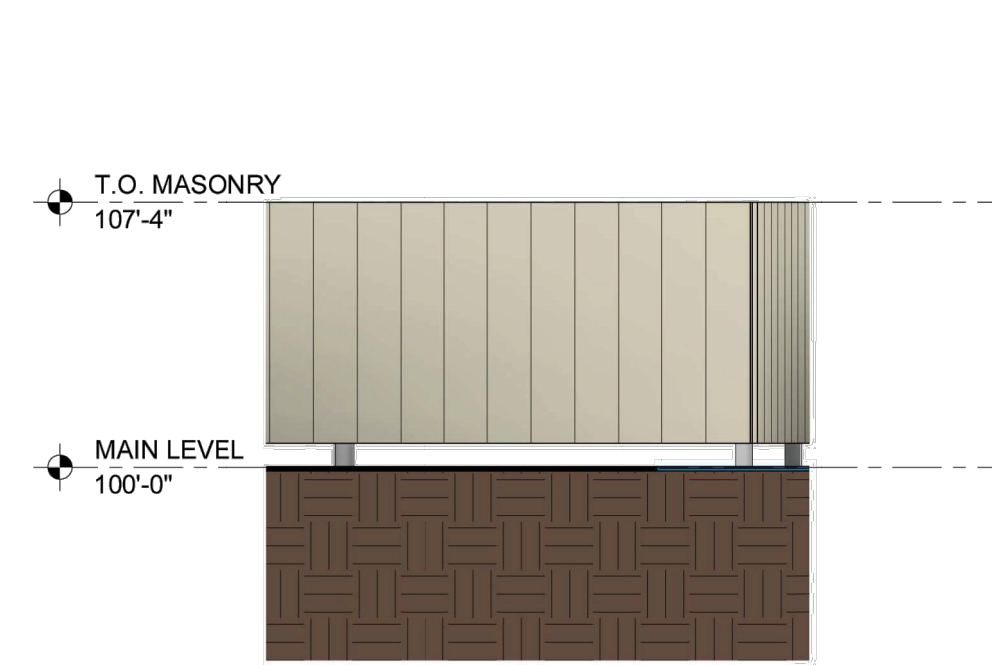
3 UTILITY FENCE - NORTH EAST SCALE: 3/16" = 1'-0"
